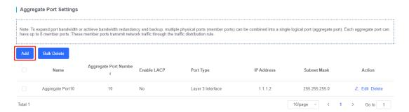
Figure 3-47 Adding an aggregated port-2
